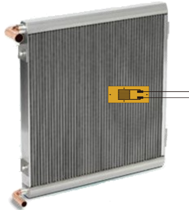
Strain gages placed near area around crack observation
